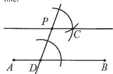
3. Construct and label a line that is parallel to the given line and passes through point P. Use geometry symbols to write a statement about the lines being parallel.
