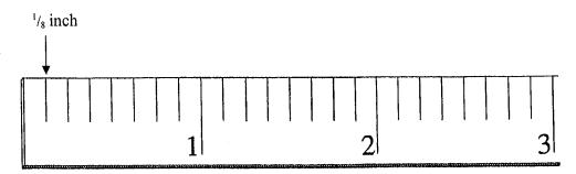
The smallest and most accurate units that an inch is divided into are  $^1/_{16}$  - inch units. There are sixteen  $^1/_{16}$  - inch units in every inch.
