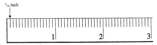
All of the units of an inch are shown on a ruler simultaneously. The vertical lines marking each unit are of varying lengths. The inch lines are the longest,  $^{1}/_{2}$  - inch lines are the second longest,  $^{1}/_{4}$  - inch lines are the third longest,  $^{1}/_{8}$  - inch lines are the fourth longest, and  $^{1}/_{16}$  - inch lines are the shortest.
