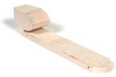
3. Smooth the corners of your car body. Use a bench-mounted sander, sharp knife, wood rasp, files, or rough sandpaper (80 grit) to smooth the car to its basic rounded shape.
